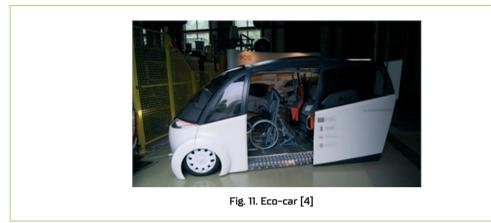
The car uses an integrated drive and brake-by-wire system, and is powered by lithium-ion batteries and a super-capacitor system. The design of the vehicle takes into account the assumptions in the ergonomic design process. The Eco-Mobility project was implemented at the Faculty of Transport of the Warsaw University of Technology.
