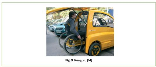
The "Kenguru" (Figure 9) is equipped with an easy-to-use scooter steering wheel, and driving it does not require a driving license [15]. The vehicle is manufactured by an American company based in Texas, KLD Energy Technologies. At the beginning of 2016, it launched a new model of a motor vehicle for a person in a wheelchair. Compared to the previous version of Kenguru, the exterior of the vehicle has been changed, the performance and the power module have been improved.
