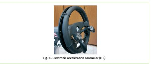
Together with the device presented above, a brake is also used, which is mounted in the form of a rod on the steering wheel.
