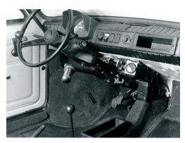
Fig. 12. The adaptation device used in the Fiat 126, RGH I car [35]
