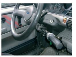
Fig. 13. RGH I adaptive device [34]
