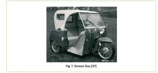
Wheel suspension on independent wishbones sprung by motorcycle shock absorbers with oil damping, rear wheels vertically stabilized with a reaction bar. The steering damper in the steering system is mounted as a Bowden cable in a closed system. The maximum speed was 55 km/h, in practice it did not exceed 60 km/h [37].
