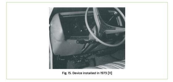
After 2000, the development of vehicles for people on wheelchairs. However, many people still use traditional vehicles incorporating a large pool of adaptive devices from companies other than car manufacturers. Acceleration is obtained by turning the lever located at its base, while in order to brake, push the lever towards the dashboard of the car.
